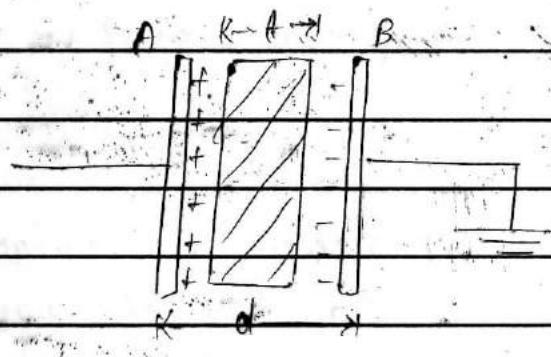
Expression: Let two parallel plate capacitor A and B with charges  $+Q$  &  $-Q$  respectively are placed  $d$  distance apart.
